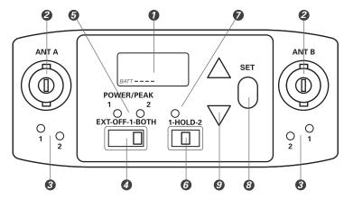
LCD 1 Liquid Crystal Display shows battery status and frequency settings. (Use the Dual-channel Control Switch (6) to select frequencies for Receiver Channel 1 and Receiver Channel 2: in Hold position, only Receiver Channel 1 frequency appears in LCD.) Battery meter is only active when Dual-channel Control Switch is in the Hold position.
